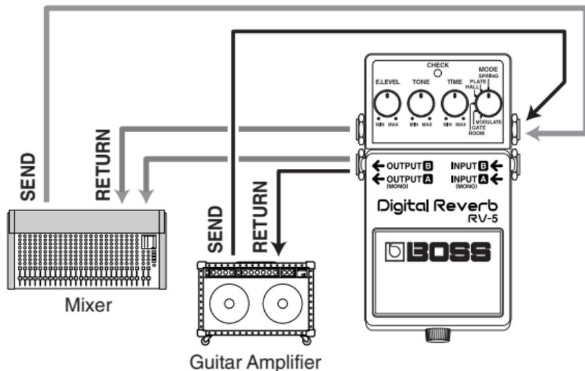
\* Make sure the input/output levels of devices being connected are matched appropriately.
