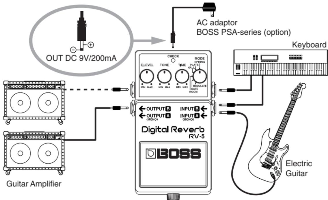
\* Be sure to lower the output level of any device being connected.
